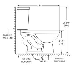
Dimensions may vary (+) or (-) 1/4". Dimensions shown in parentheses are in millimeters: 25.4 mm = 1 inch. Note: Fixture dimensions are nominal and conform with dimension and performance requirements of ASME/ANSI Standards A112.19.2M. PSI rating: 20 minimum to 80 maximum per ASME A112.19.2. Dimensions subject to change or cancellation without notice. Briggs is not responsible for the use of superseded or voided specification information.
